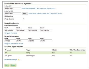
Figure 5. Computing the Bounding Box
