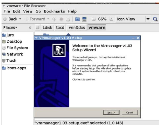
Figure 1. VMmanager should run under Wine in Unix (you see installation in GNOME)
