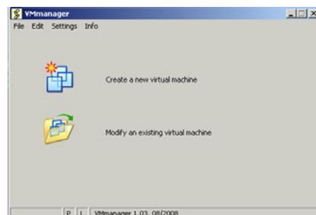
Figure 2. With VMmanager you can create a new VMware image, or edit the existing configuration of virtual disks
